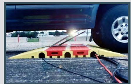
The system's high-powered pulse causes the targeted vehicle's electronics to malfunction temporarily without harming its occupants.
