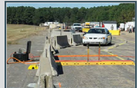
PEVS stops vehicles at significant keep-out ranges, reducing risk to personnel from vehicle-borne improvised explosive device blast effects
